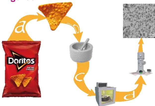
**Figure 1.** Full process to separate the nanomaterial from the food product: a. product selection; b. sample preparation; c. matrix digestion; d. characterization. TEM image: SiO<sub>2</sub> nanoparticles extracted from Doritos.
