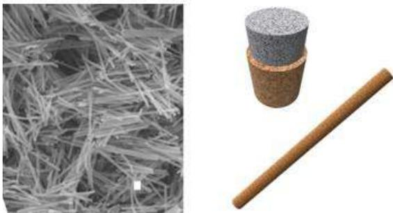
**Figure 1.** Ni@Au NWs: Ni NWs fabricated by templated assisted electrodeposition and covered with a gold layer by galvanic displacement in a Au(III) solution. Scale bar: 200 nm
