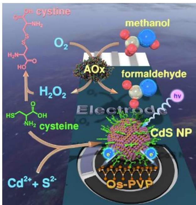
Figure 4. Photo-electrochemical bioassay for methanol.
