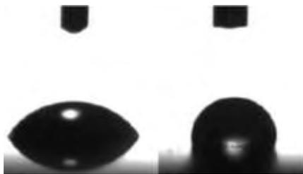
Figure 3. Contact angle measurement of a flat sample coated (left) and uncoated (right): a decrease in contact angle after coating is observed, which means an increase in wettability.
