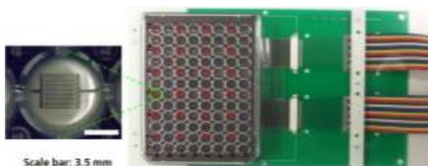
**Figure 1.** The sensor in well plate format is connected to a circuit board. The ribbon cables lead to the measuring device. On the left an enlarged picture of one well with an interdigital structure is shown.
