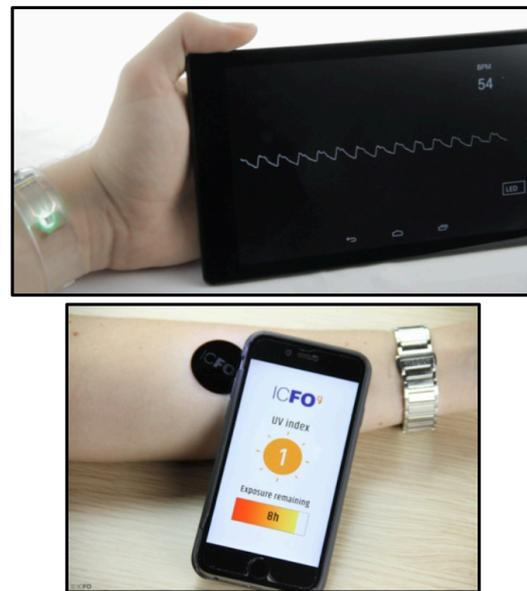
**Figure 1.** (a) Graphene based flexible and transparent wellness sensing platform.(b) Battery-less UV monitor powered via NFC communication.
