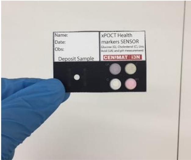
Figure 1. Real-size image of paper-based, 3D multiplex platform for screening of glucose, cholesterol and uric acid.
